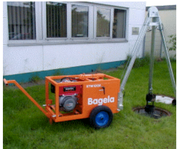
KTW 1005 with wheels, tow bar and triple beam (extra accessories) for sewer cleaning jobs.
